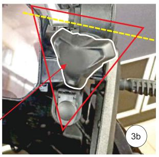
**4.** Motor is supplied with a red pin installed to determine the position. Now you can attach the GearBox to the **triangular knob** to raise and Lower the windshield as follows:
