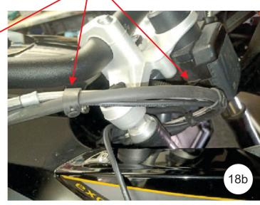
19. Installation of the electrical wiring and of the Power Y- connector:
