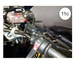
12. Install the Switch Button over the mirror perch
