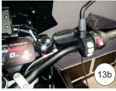
14. The switch can also be installed on the left mirror perch if desired.
