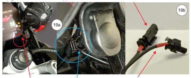
Unplug the connector from the auxilliary power socket and install the Power Y-Connector inbetween
