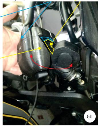
7. Screw the lower Allen M6 screw at the windshield lift mechanism to secure the GearBox
