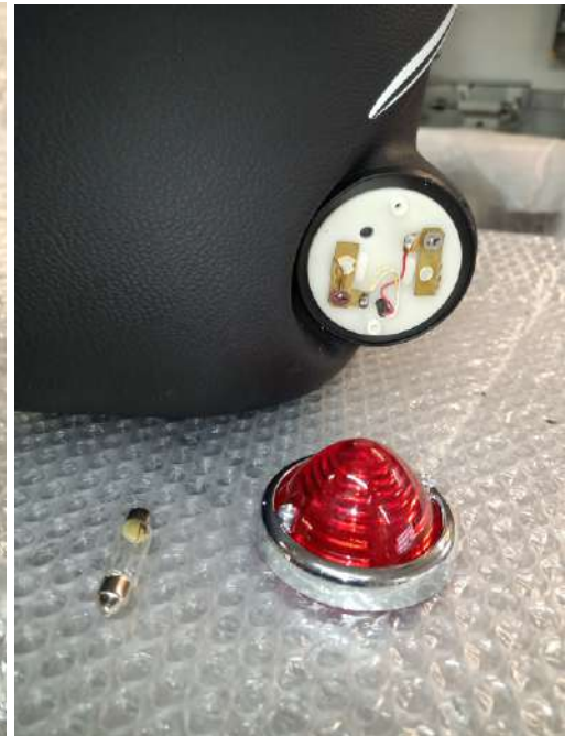
Attach the lamp housing and drill a 5 mm hole for the power cable
