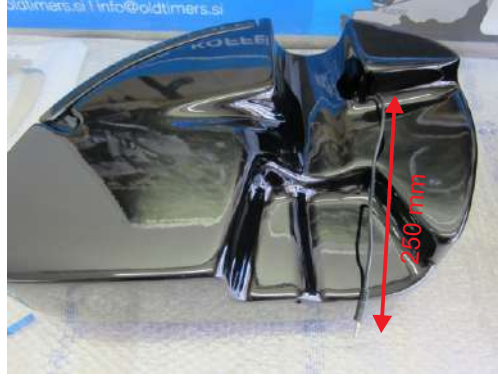
Attach the lamp housing and drill a 5 mm hole for the power cable
